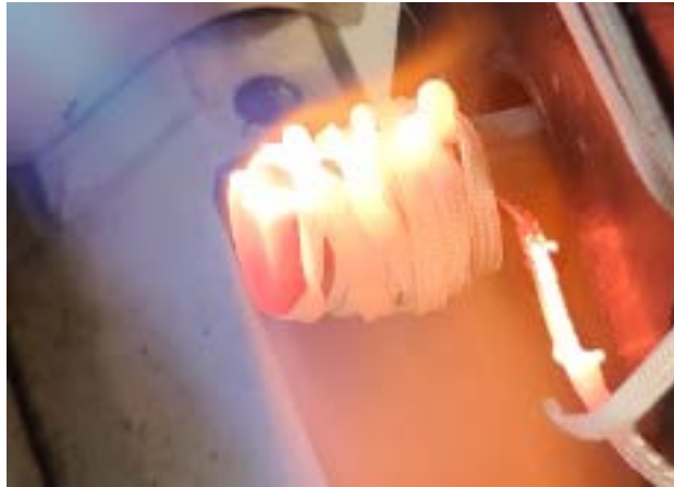
Figure 7. Probe and a thermocouple heated to 1100 °C
